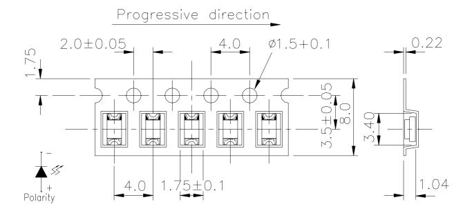
**Note:** Tolerances Unless Dimension is  $\pm 0.1$ mm, Unit = mm
