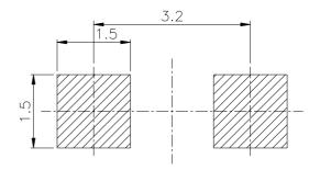
**Note:** Tolerances Unless Dimension is  $\pm 0.1$ mm, Unit = mm
