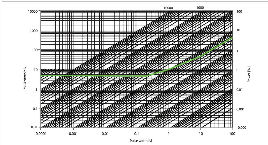
Pulse power for continuous operation.
